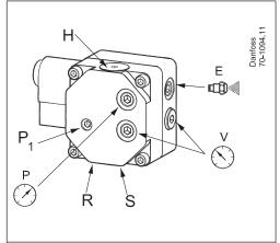
P<sub>1</sub>: Pressure adjustmentS: Suction inlet G 1/4
