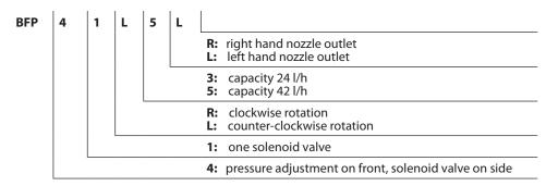
Nozzle capacity at 4.3 cSt., 10 bar, 2800 min-1
