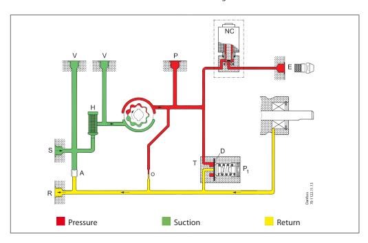
From the suction inlet (S) oil is drawn through the filter (H) to the gear set, where the pressure is increased. When voltage is applied to the NC-valve (normally closed), it opens and releases oil to the nozzle outlet.
